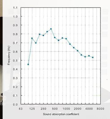
These measurements meet the requirements of ISO 354.All measurements were carried out on standard boards with acoustic tissue laminated on the back.
